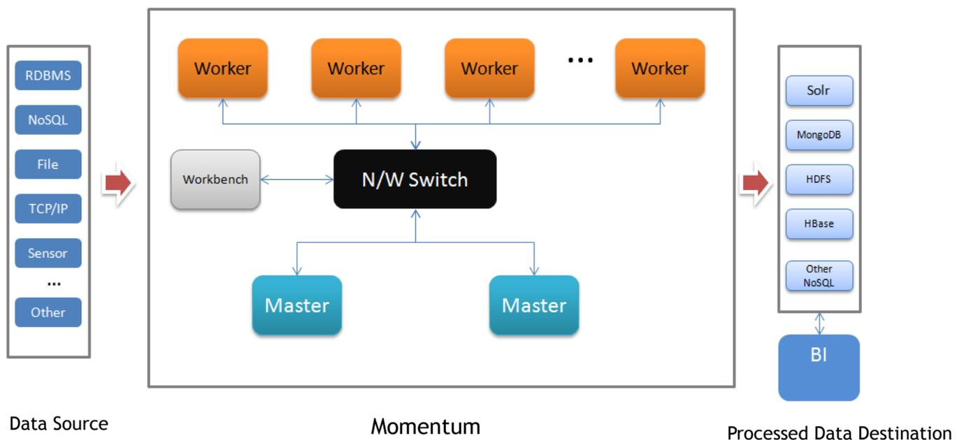
Momentum is a cluster based technology with master-slave architecture as shown in the above diagram.
